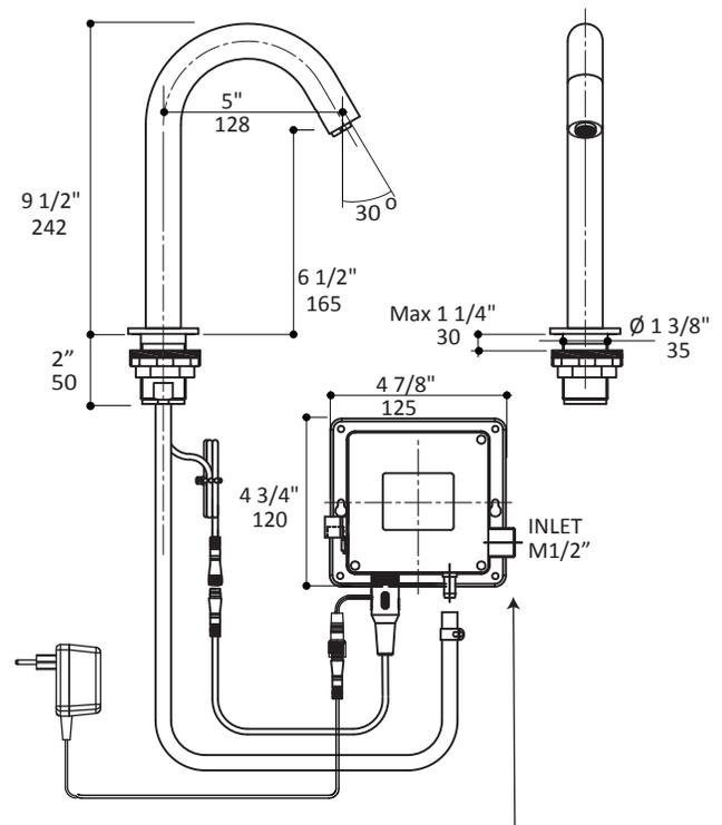
**IMPORTANT:** Install provided flow reducer on the water inlet
