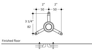
In-floor plumbing connections 2 x 1/2" copper pipe
